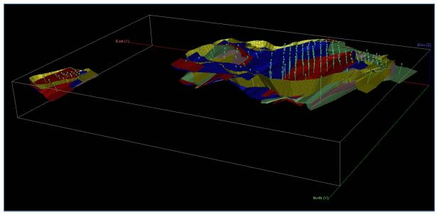
1. All mineralized zones are shown (different colors), as are drill holes (blue) and the pit shell (yellow).
