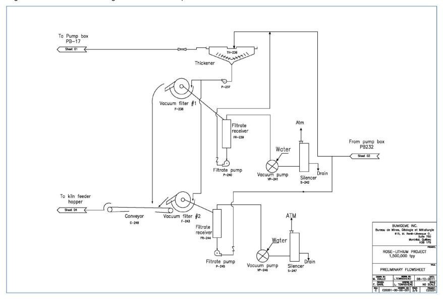
Figure 17-3 Flowsheet Diagram – Sheet 3/5 – Spodumene Concentrate Filtration Circuit.
