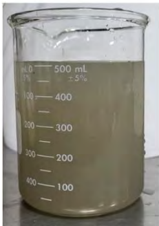
Figure 13.11: Spodumene Concentrate - Filtrate Quality
