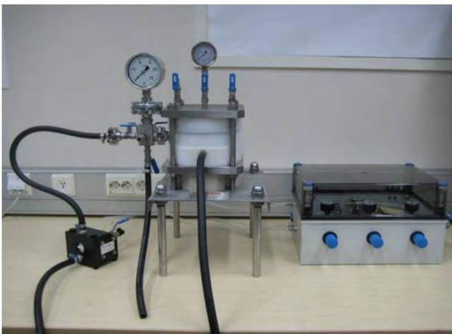
Figure 13.9: Labox 100 Test Unit in PF Orientation as Tested
