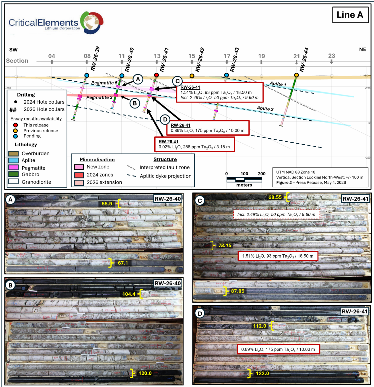
Figure 2: Vertical section – Line A; looking northwest
