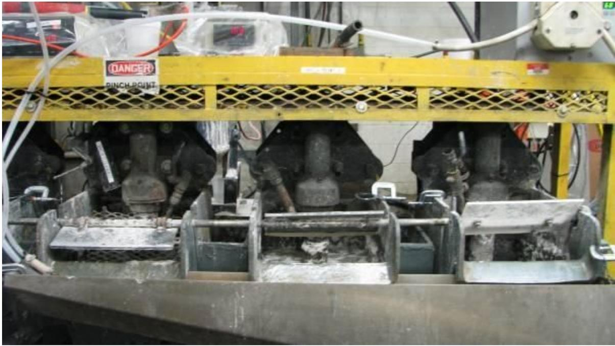
**Figure 5 - Mica Flotation Cells**
