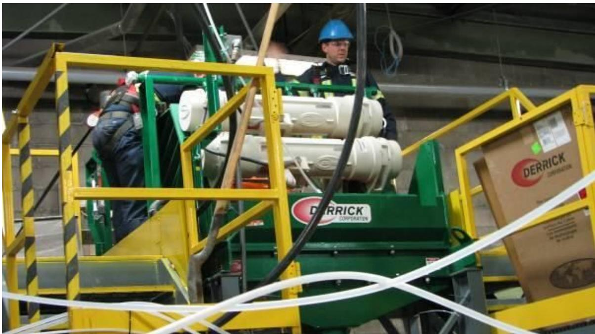
Figure 2 - Ball Mill & Derrick Screen. Overs from Derrick feed Ball Mill
