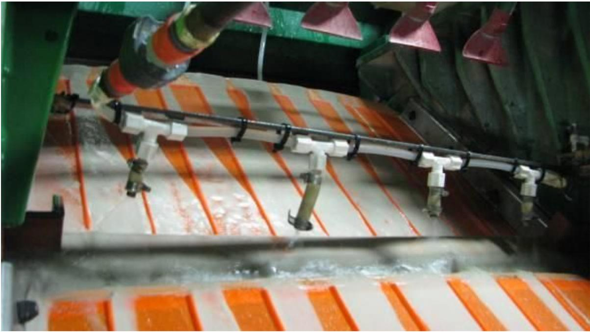
Figure 3 - Derrick Screen with mineralized material
