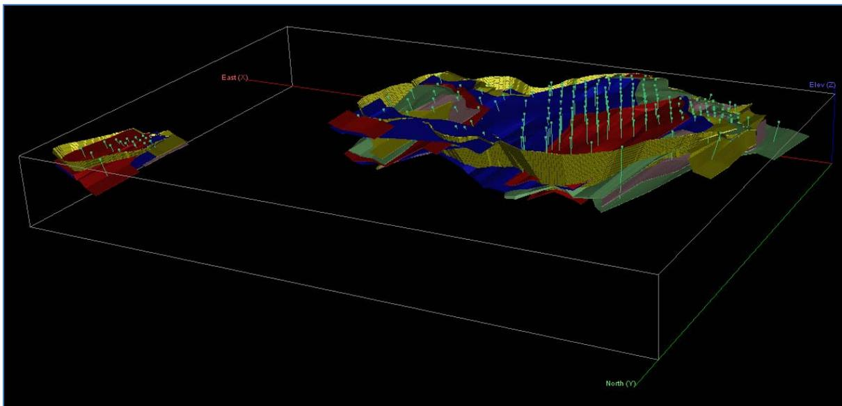
1. All mineralized zones are shown (different colors), as are drill holes (blue) and the pit shell (yellow).
