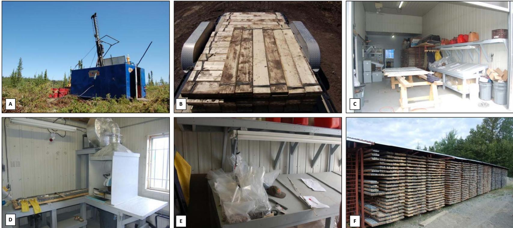
1. A) Drill rig on the Rose deposit; B) Core carefully boxed and ready for transport by Consul-Teck personnel to the Val-d'Or facility; C) Consul-Teck logging facility where the core is logged and marked for sampling; D) Core splitter used to sample the core; E) Half-core bagged by Consul-Teck personnel and later shipped to the assay laboratory; F) Core adequately stored outside in roofed-racks. Photos taken by author P.-L. Richard during his visit of the property and Val-d'Or facilities.
