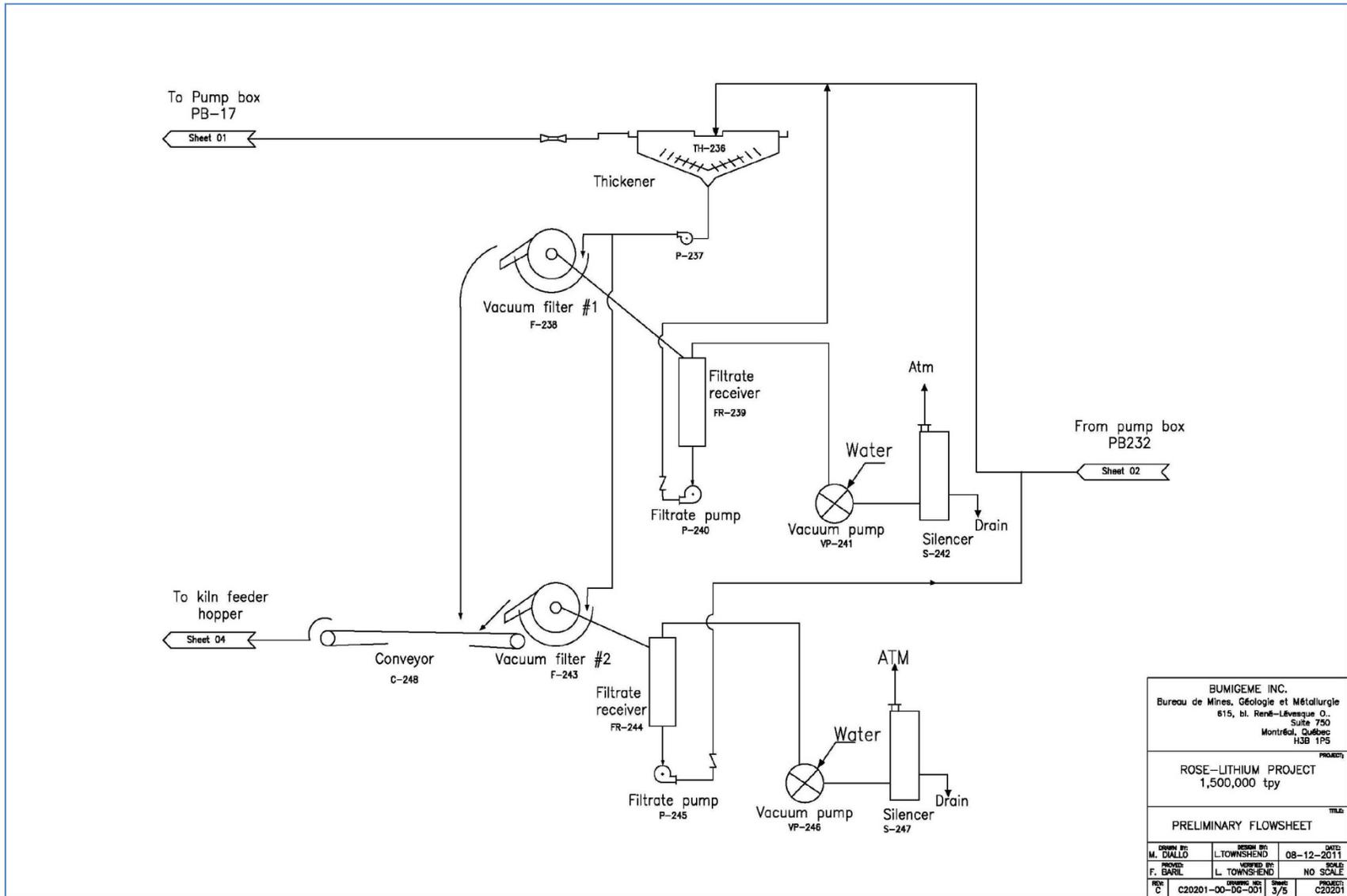
Figure 17-4 Flowsheet Diagram – Sheet 4/5 – Lithium Carbonatation Circuit.
