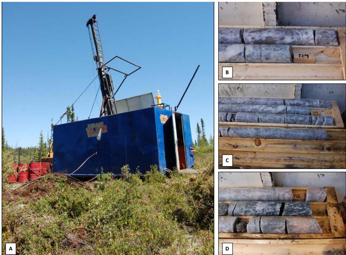
1. A) Drill rig in action on hole LR-10-86 at the time of the field visit; B) to D) Views of the Rose pegmatite in core that was drilled in the author's presence. Photos taken by author P.-L. Richard
