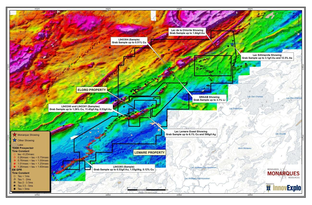
Figure 26.1 – Airborne magnetic survey showing the main anomalies on the Lemare property
