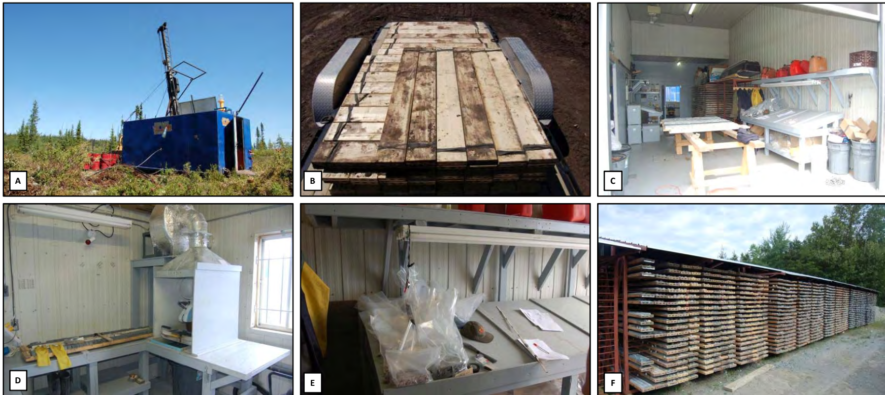
Figure 12.6 – Path of the core from drill rig to final storage facility: A) Drill rig on the Rose deposit; B) Core carefully boxed and ready for transport by Consul-Teck personnel to the Val-d’Or facility; C) Consul-Teck logging facility where the core is logged and marked for sampling; D) Core splitter used to sample the core; E) Half-core bagged by Consul-Teck personnel and later shipped to the assay laboratory; F) Core adequately stored outside in roofed-racks. Photos taken by author P.-L. Richard during his visit of the property and Val-d’Or facility.
