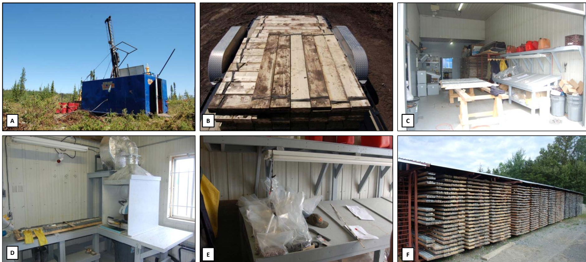
Figure 14.4 – Path of the core from drill rig to final storage facility: A) Drill rig on the Rose deposit; B) Core carefully boxed and ready for transport by Consul-Teck personnel to the Val-d’Or facility; C) Consul-Teck logging facility where the core is logged and marked for sampling; D) Core splitter used to sample the core; E) Half-core bagged by Consul-Teck personnel and later shipped to the assay laboratory; F) Core adequately stored outside in roofed-racks. Photos were taken by the author during his visit of the property and the Val-d’Or facility.
