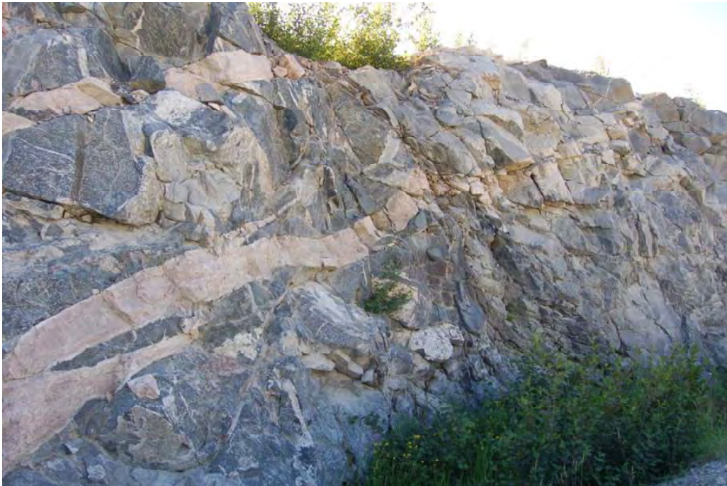
Figure 9.5 – Example of another pegmatite occurrence in the vicinity of the Rose and Pivert showings (in this case, a road cut). The photo shows a pegmatite in which molybdenite and spodumene were noted. Note that the pegmatite cuts through a deformation zone without showing any signs of being affected by it. Photos taken by the author during the field visit.
