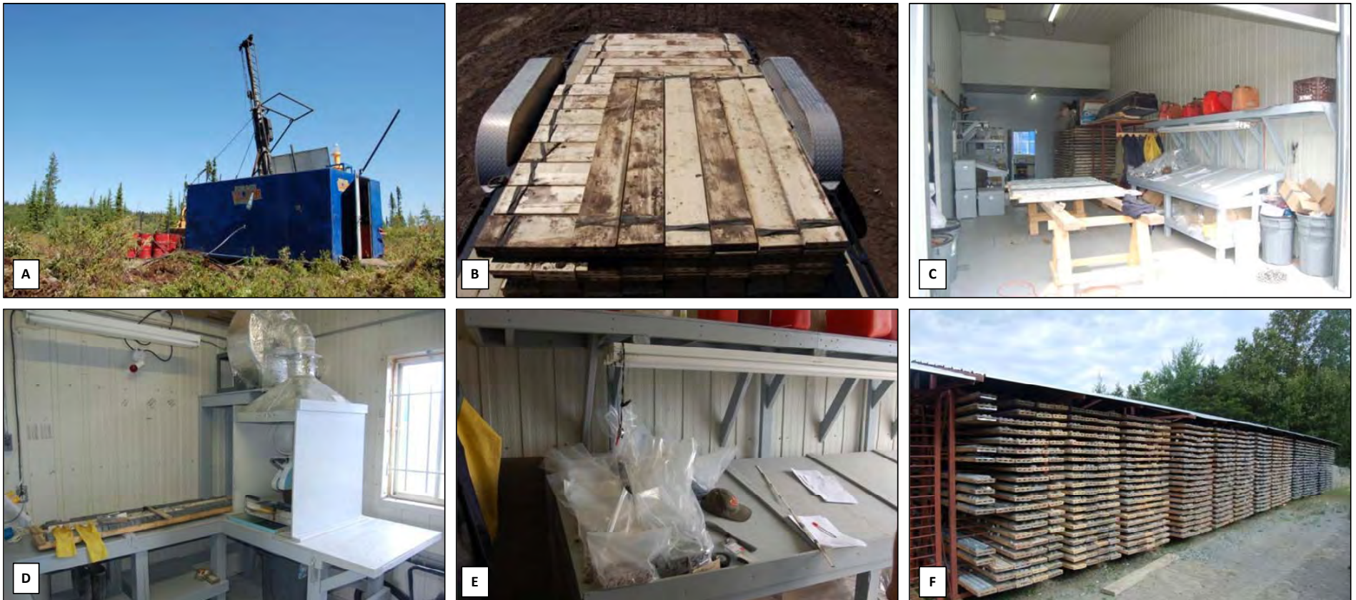
Figure 14.4 – Path of the core from drill rig to final storage facility: A) Drill rig on the Rose showing; B) Core carefully boxed and ready for transport by Consul-Teck personnel to the Val-d’Or facility; C) Consul-Teck logging facility where the core is logged and marked for sampling; D) Core splitter used to sample the core; E) Half-core bagged by Consul-Teck personnel and later shipped to the assay laboratory; F) Core adequately stored outside in roofed-racks. Photos were taken by the author during his visit of the property and the Val-d’Or facility.
